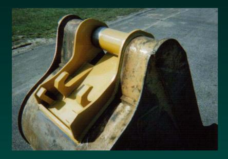
THE CONVERSION BLANK IS THEN WELDED IN PLACE
